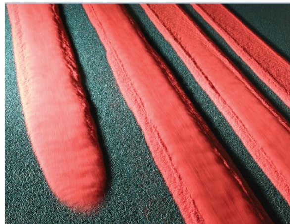
Fig. 2 Small scale self-channelized flows of mono-disperse red sand on a rough inclined plane (Rocha et al. 2019). Note the formation of static levees.
